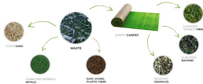
Figure 19: 100%TurfRecyclers' "from waste to resource" process
